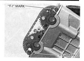
If the timing marks are facing outward, turn the crankshaft counterclockwise 3/4 turn (270°) and align the "RT" mark with the index mark.
