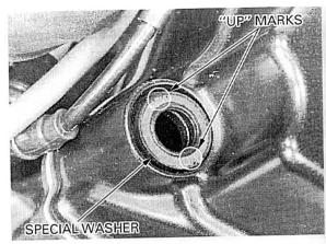
Install and tighten the cylinder head cover bolts.
