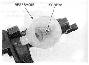
Remove the screw and clutch switch. Remove the pivot nut, bolt and clutch lever assembly.
