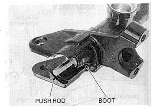
Apply silicone grease to the push rod hole in the clutch lever joint piece.
