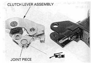
Apply silicone grease to the pivot bolt sliding surface and install the bolt into the master cylinder and clutch lever.
