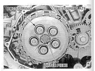
Remove the clutch lifter rod from the mainshaft. Remove the clutch discs, plates, judder spring and spring seat.
