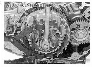
Remove the special washer and clutch center.
