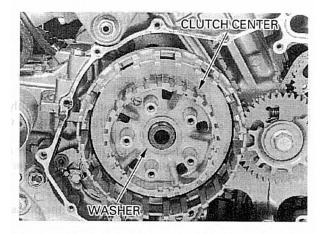
Remove the thrust washer.
