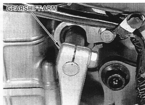
Remove the gearshift spindle assembly and thrust washer.
