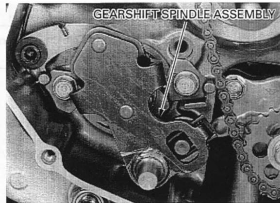
Remove the gearshift cam bolt and gearshift cam.
