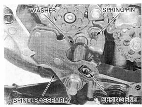
Install the gearshift arm onto the spindle, aligning the slit of the arm with the punch mark on the spindle.
