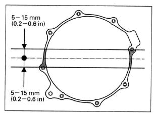
Install the dowel pins and a new gasket.
