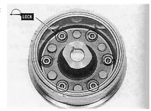
Install the starter driven gear while turning it counterclockwise.
