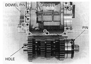
Install the mainshaft assembly, aligning the hole in the needle bearing outer race with the dowel pin.
