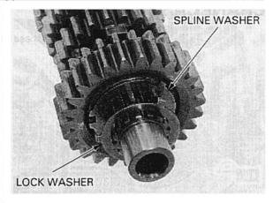
Install the countershaft assembly, aligning the hole in the needle bearing outer race with the dowel pin, and the set ring with the ring groove.
