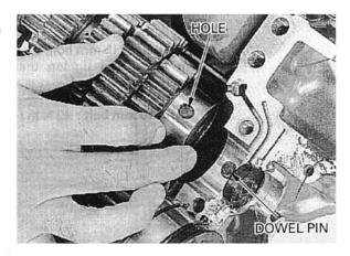
Apply locking agent to the set plate bolt threads. Install the mainshaft bearing set plate with the "OUT SIDE" mark facing out and tighten the bolts.
