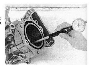
Calculate the cylinder taper and out-of-round at three levels in an X and Y axis. Take the maximum reading to determine the taper and out-of-round.
