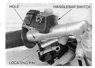
Install the clutch master cylinder and holder with the "UP" mark facing up.
