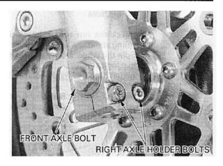
Loosen the left front axle holder bolts. Remove the front axle and the front wheel.
