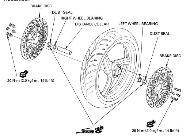
Drive in a new left bearing squarely with the marking side facing up until it is fully seated. Install the distance collar.
