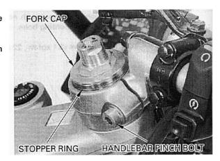
Loosen the fork top and bottom pinch bolts, and remove the fork tube from the fork bridges.
