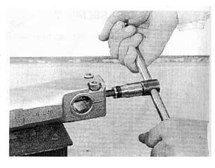
Remove the fork damper, rebound spring and oil lock piece from the fork tube.
