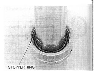
Apply fork fluid to a new dust seal lip and install the dust seal into the fork slider.
