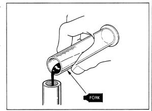
Pump the damper rod several times until the fork fluid flow out of the oil hole in the rebound damping adjuster.
