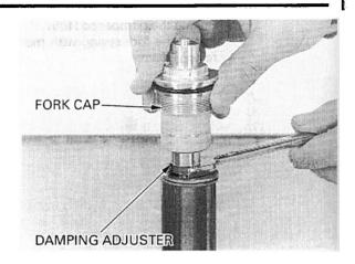
Install the fork cap into the fork tube.
