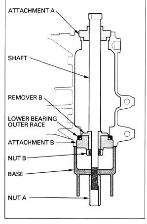
Install a new upper bearing outer race and the ball race remover as shown.
