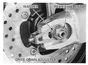
Push the rear wheel forward and derail the drive chain from the final driven sprocket.
