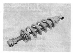
Remove the lower joint pivot collar. Check the dust seals and needle bearing for wear or damage; replace them if necessary.
