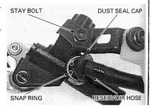
Remove the pivot nut, bolt and brake lever assembly.
