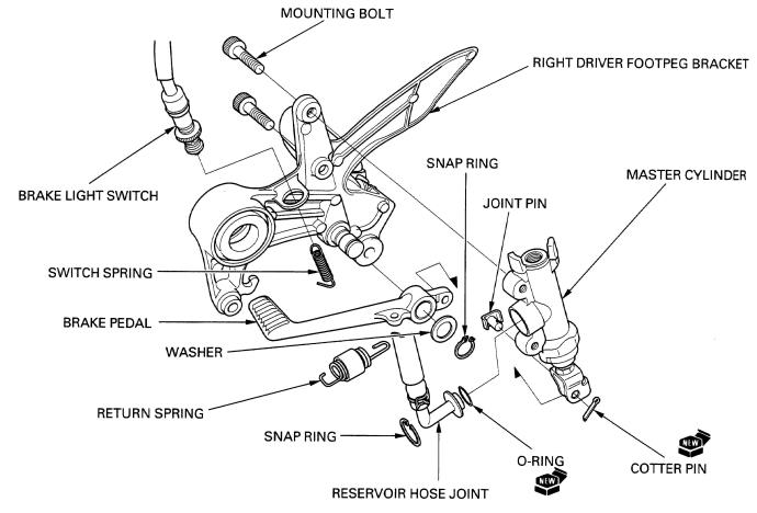
Coat the master piston and piston cups with clean brake fluid.
