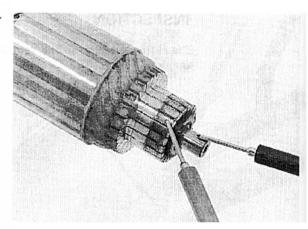
Check for continuity between the insulated brush and cable terminal.
