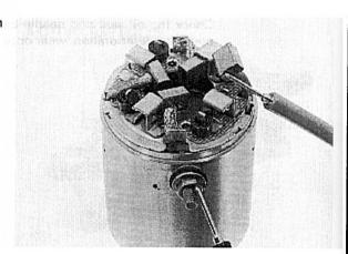
Check for continuity between the insulated brush and motor case.
