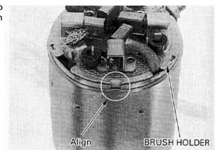
Push and hold the brushes inside the brush holder, and install the armature through the motor case and brush holder.
