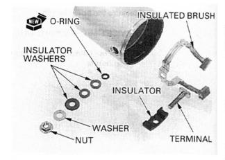
Install the brush holder, aligning the holder tab with the case groove, and the holder grooves with the insulated brush wires.
