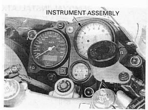
Pull the socket out of the instrument case.
