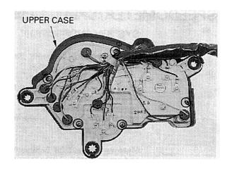
Remove the screws, speedometer, tachometer and coolant temperature gauge.
