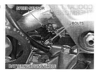
Coat a new O-ring with oil and install it onto the speed sensor.
