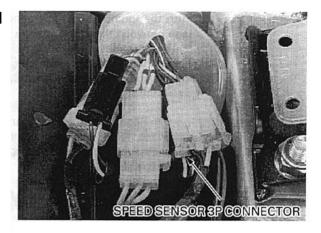
Remove the two bolt, battery ground cable and speed sensor.
